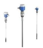
**Liquicap M FMI52:** This instrument is used for continuous level measurement in liquids. It uses capacitive sensor technology and as long as the liquid has a conductivity  $>100\mu S/cm$  no calibration is necessary. The unit operates from -80 to  $200^{0}C$  in the medium container and from a vacuum to an over pressure of 100 bar. The units come calibrated to the ordered probe length from the factory, allowing easy commissioning. The FMI52 is also suitable for interface measurement.
