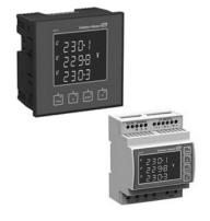
**RV12 and RV15 Energy meters:** Designed for low voltage systems (up to 500V L-L or 289V L-N) these power meters are able to record, display and transmit electrical parameters such as voltage, current, frequency, THD, power factor, active and reactive power. The RV12 is top-hat rail mounted and the RV15 is a panel mounted unit. They can be used for single phase, three phase 3 wire or three phase 4 wire systems.
