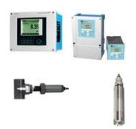
**Turbidity:** Sensors are available in measuring ranges of 0.00 to 9999 FNU or 0.0 to 300 g/l for applications ranging from monitoring in sewage plants to drinking water. The CUS65 uses a 4-beam alternating method of measuring turbidity so they are not sensitive to the aeration systems used in sewage treatment. The CUS41 measures at a 90° scattered light angle using infrared light allowing it to be insensitive to the effects of colour or dyes.
